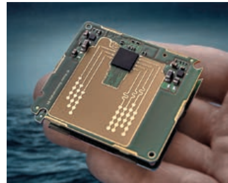
Frontend for a high-resolution radar system with AI support for processing data for cooperative autonomous driving
