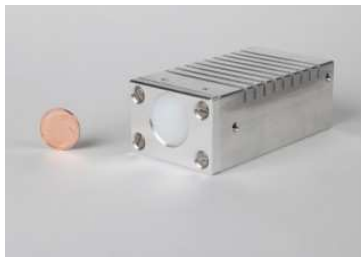
Miniature RADAR sensor in W-Band
