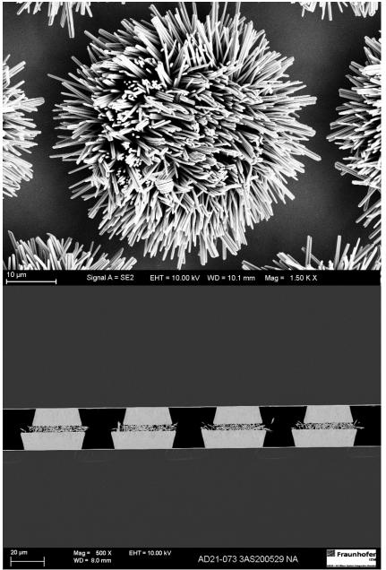
Groundbreaking interconnection technology using 200 nm nanowires to realize tomorrow's high-performance electronics. I © Fraunhofer IZM I Print quality images: www.izm.fraunhofer.de/pics
