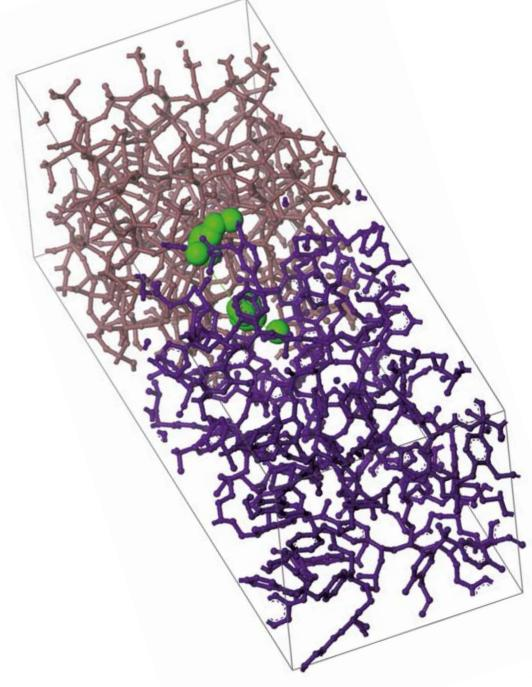
Profile of movement of a single water molecule at the interface of epoxy/SiO<sub>2</sub>
