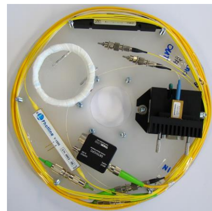
Experimental fiber optic gyroscope setup for testing issues of components, e.g. fiber depolarizer, air fiber coil, integrated beam splitter
