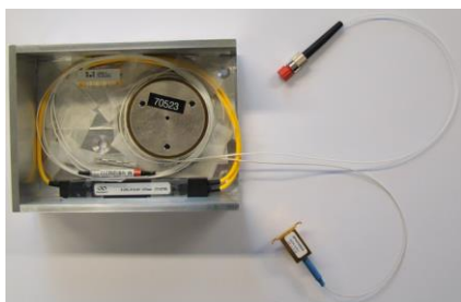
Space grade fiber optic gyroscope based on standard components
