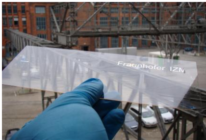
Thin glass sheet with integrated waveguides.
