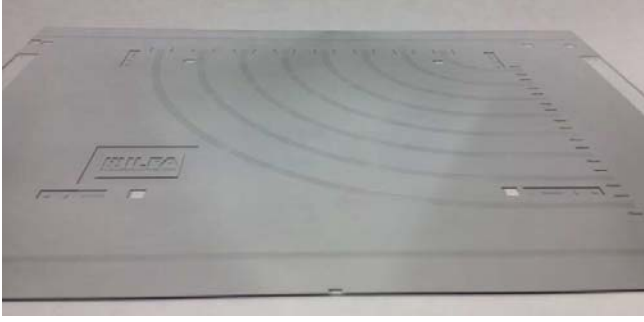
Figure 8. Glass panel 220 mm x 285 mm with diffusion mask after laser separation.
