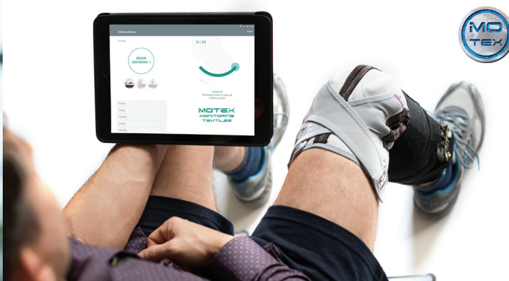
Knee brace with textile stretch sensor for therapeutic monitoring
