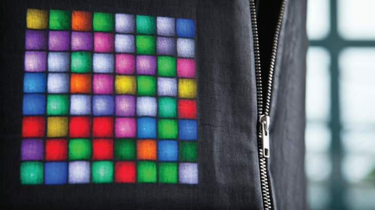
Smart pixel display bonded to a woven circuit substrate
