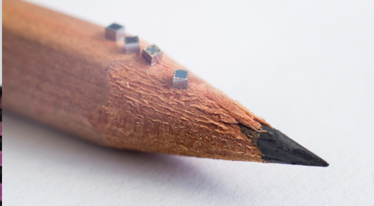
Piezoresistive silicon pressure sensors
