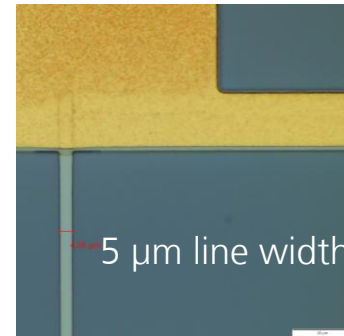
Niobium patterned: 50 µm down to 5 µm line width & electroplated Au 1.5 µm
