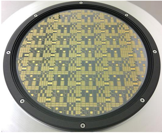
8" wafer: Nb 150nm / Au 150nm; electroplated Au: 1.5µm
