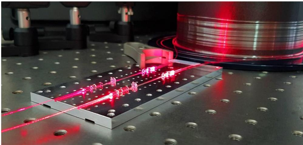
**The use of hollow-core fibers makes fiber optic gyroscopes less susceptible to external interference factors. | © Fraunhofer IZM Druckqualität:**
