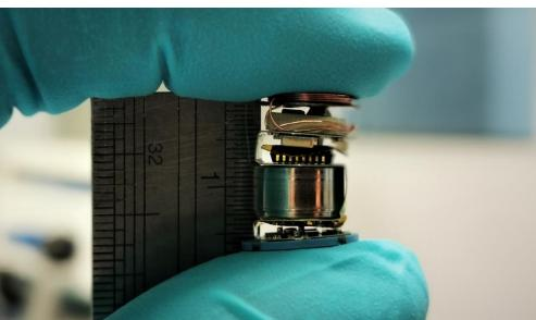
The core of the spectroscopy capsule contains the system-in-package, a flexible circuit board, and a ceramic pcb
