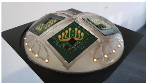
The polyurethane ceiling unit equipped with four radar modules.
