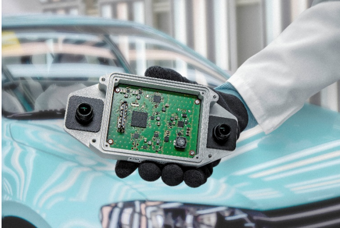
Picture 1: A shot of the camera/radar module with its housing.
