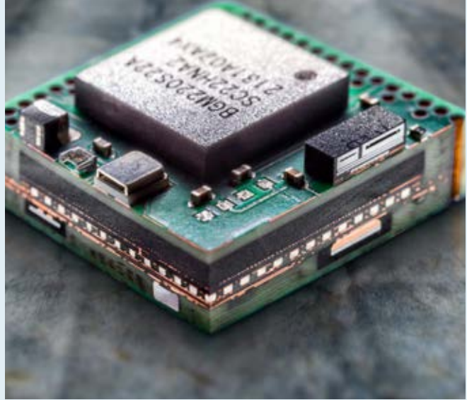
Embedded highly miniaturized sensor and controller module
