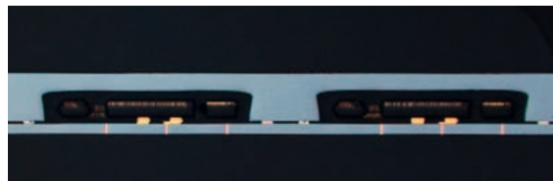
Hermetic sealing by bonding a cap wafer to a TSV device wafer
