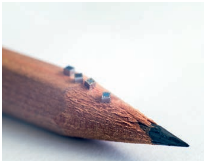
Piezoresistive pressure sensor with 0.8 mm 2 footprint
