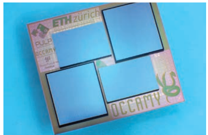
Silicon interposer with two accelerator compute units and two high bandwidth memory (HBM) stacks for high performance computing (Chip/system design: ETH Zurich, interposer finish and chip assembly: Fraunhofer IZM)
