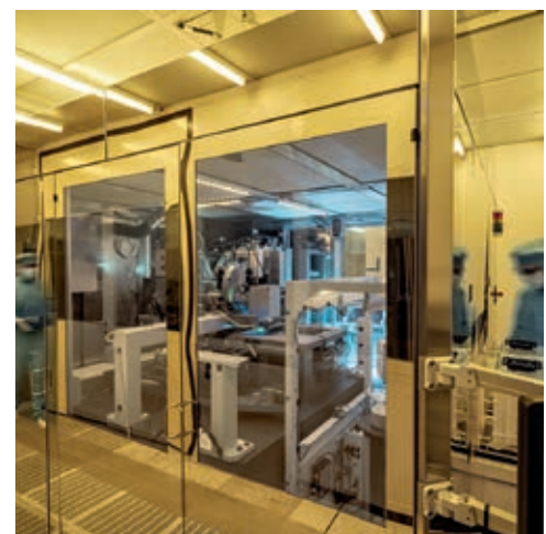
Wafer process line up to 300mm
