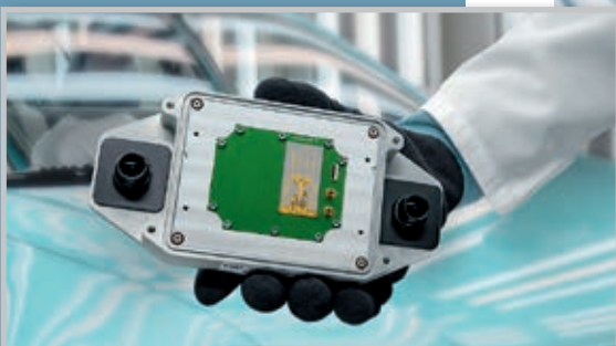
Radar sensor module for autonomous driving
