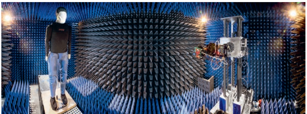
Measurement of a radar module for use in security technology with a 79 GHz dummy
