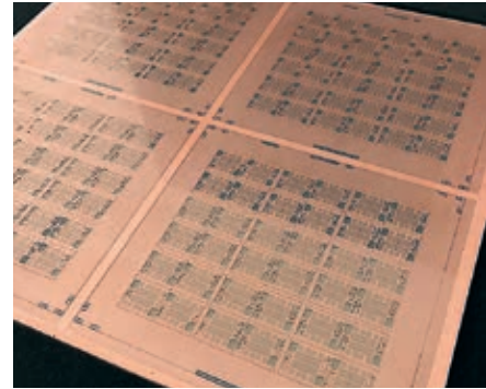
Prototype of a glass core substrate, 510mm x 515mm, manufactured in preliminary tests at Fraunhofer IZM
