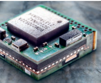
Highly miniaturized edge-IOT-module
