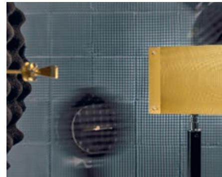
Surveying of intelligent reflective surfaces (IRS) for 6G applications
