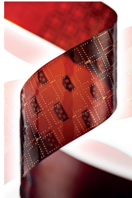
Flexible Multi-Layer Substrate with High Density Copper Wiring
