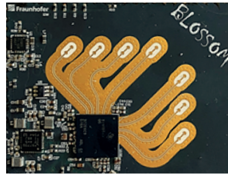
Design of the radar module based on an IWR6843-TI chip
