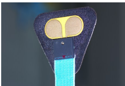
Laminated textile-integrated capacitive EMG sensor for measuring muscle activity in an unobtrusive way
