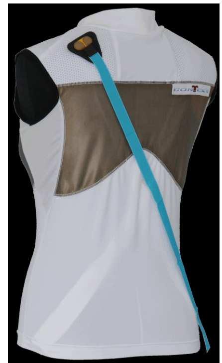
Final prototype vest with EMG sensor placed on the outside for better visibility of the technology
