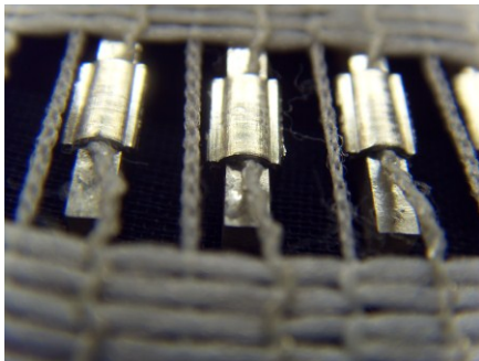
Crimped textile-integrated insulated wire
